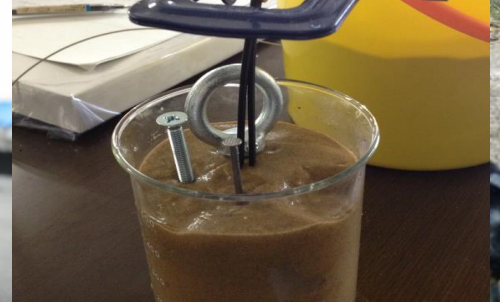
Liquefaction (Movements of sand particles in water)
